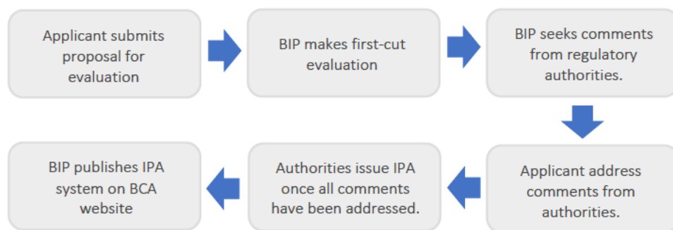
Figure 7: Building Innovation Panel PPVC acceptance process (adapted from BCA (2022))
